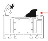
Fit a 17mm Frame Wedge to the outer frame on the stay fixing area
